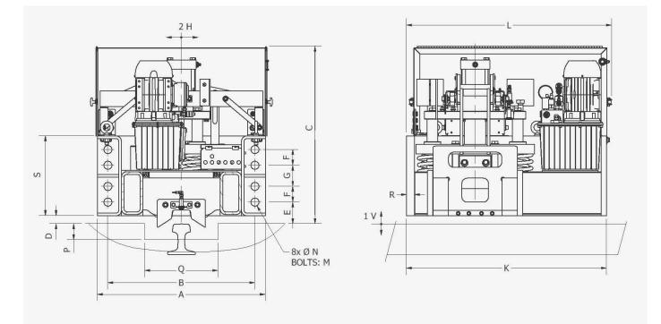
1V Vertical Rail Deviation (Float) ±25mm relative to Rail Clamp enclosure at full rated capacity.
